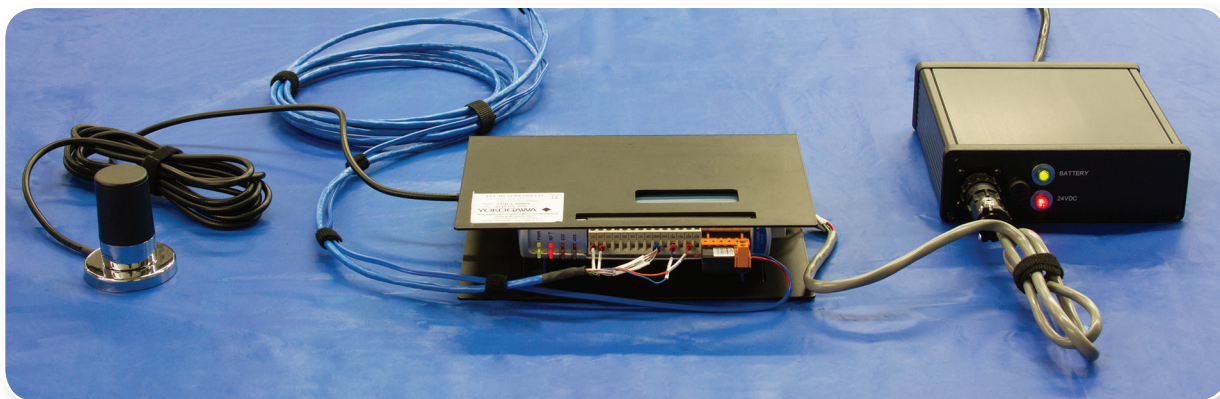
Figure 2: Each individual ultra-low freezer has a group of devices installed, including a wireless module, antenna and power supply that works together to collect data from an array of sensors and sends it back to the central monitoring and control system through the network.
