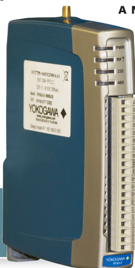
Figure 3: The basic DAWN module connects directly to the sensors through the I/O terminals. It interfaces with the larger network regardless of its location within the campus.
