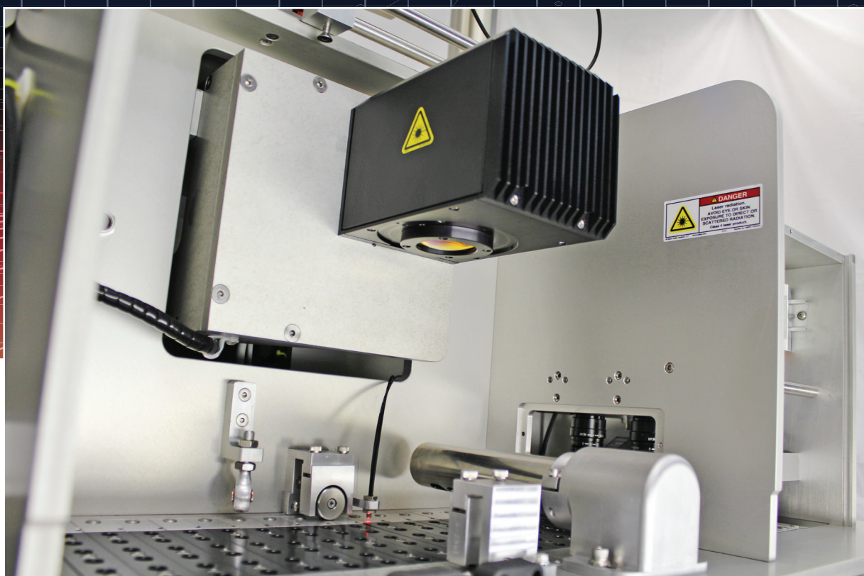
Laser in place to inspect tablets as they are conveyed to their next processing step.
