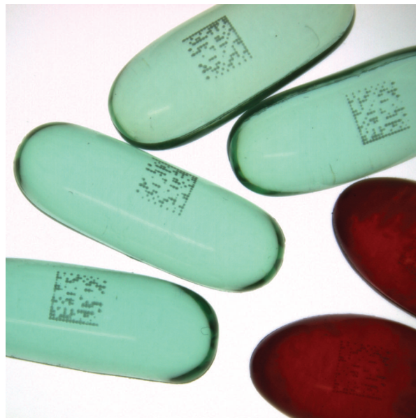
Data-matrix code, laser-inscribed on gelcaps with encrypted manufacturing information. Images courtesy of PhotoScribe.
