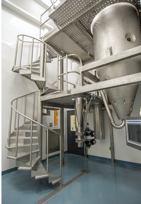
This development spray dryer is used to scale up to the same size commercial dryer in the manufacturing facility.
