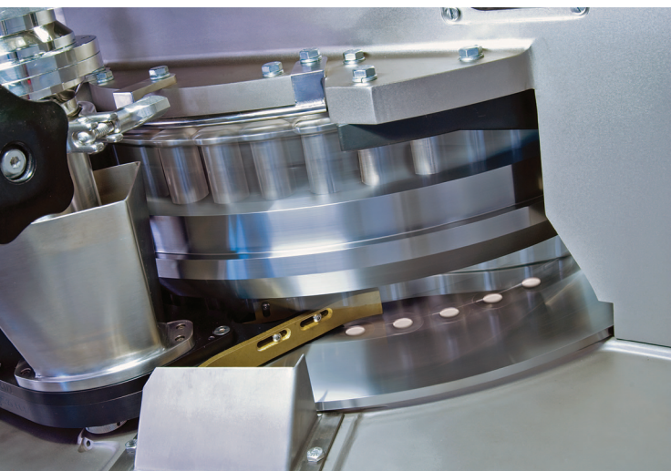
Natoli's rotary tablet press can deliver up to 5,500 tablets per minute with increased size and weight.
