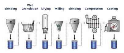
Figure 1: Batch Manufacturing<sup>4</sup>
