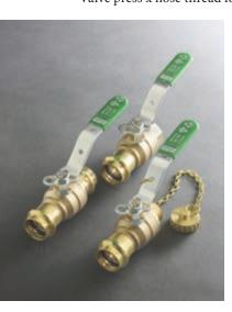
ball valves are full port and designed for potable water applications. They are available in 1/2" and 3/4" press sizes and 3/4" hose sizes. Other features include a lockable metal handle, stainless-steel ball and EPDM sealing element. The Viega ProPress for copper system is available in more than 600 fitting configurations, in sizes ranging from 1/2" to 4". The Smart Connect feature ensures the integrity of connections. VIEGA
