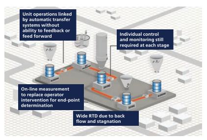
Figure 2: Automated Batch Processing
