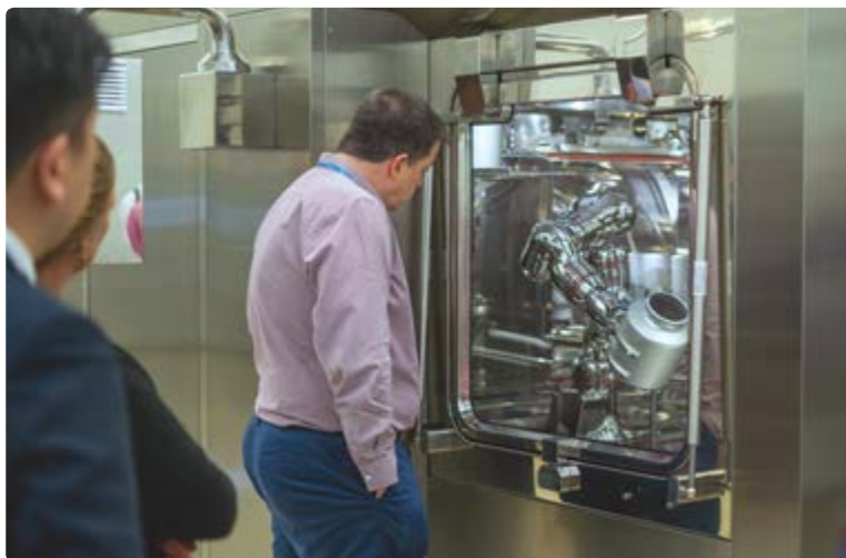
Fedegari’s new washer sterilizer features a cluster tool concept with a gloveless robotic isolator suitable for multiple formats and various batch sizes.
