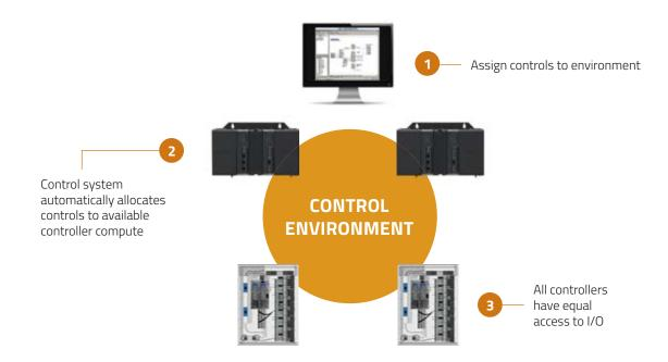
automation vendor can consolidate data and move control to a centralized local or remote data center in a private cloud. The resulting "digital twin" of the control process allows for testing of new recipes and qualification of changes to the automation system offline. The enabler is batch execution located in the controller.
