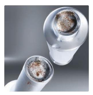
Corrosion on tablet tooling can delay production, reduce efficiency and cause contamination problems.
