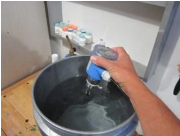
Figure 2: In a "bucket test," a level switch is removed from the vessel and immersed in material from the process to test that it switches properly.
