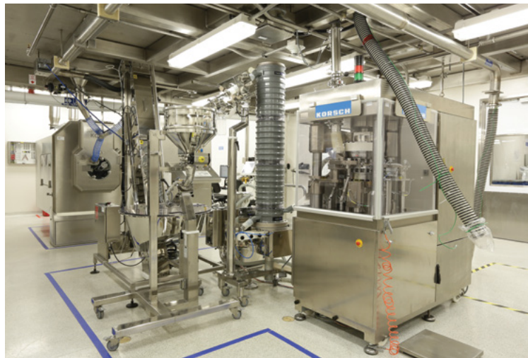
Several operations are necessary to get Prezista from mixing and blending to final tablet form. Tablet press and dedusting operations shown here.
