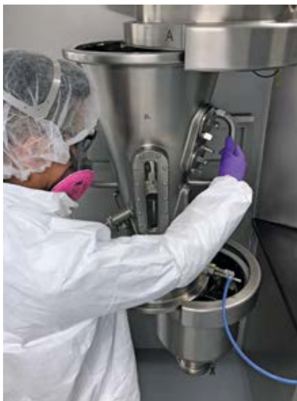
An Avista Pharma manufacturing technician removes the fluid bed multi-particulate coating insert to prepare for a top spray granulation process.
