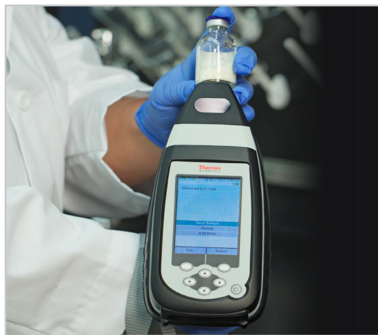
The Thermo Scientific MicroPHAZIR can provide raw material identification in seconds.
