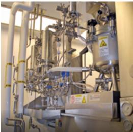
Shown here: the redundant sterile filtration and buffer tank that feeds the fill nozzles on the inside of the BFS machine.
