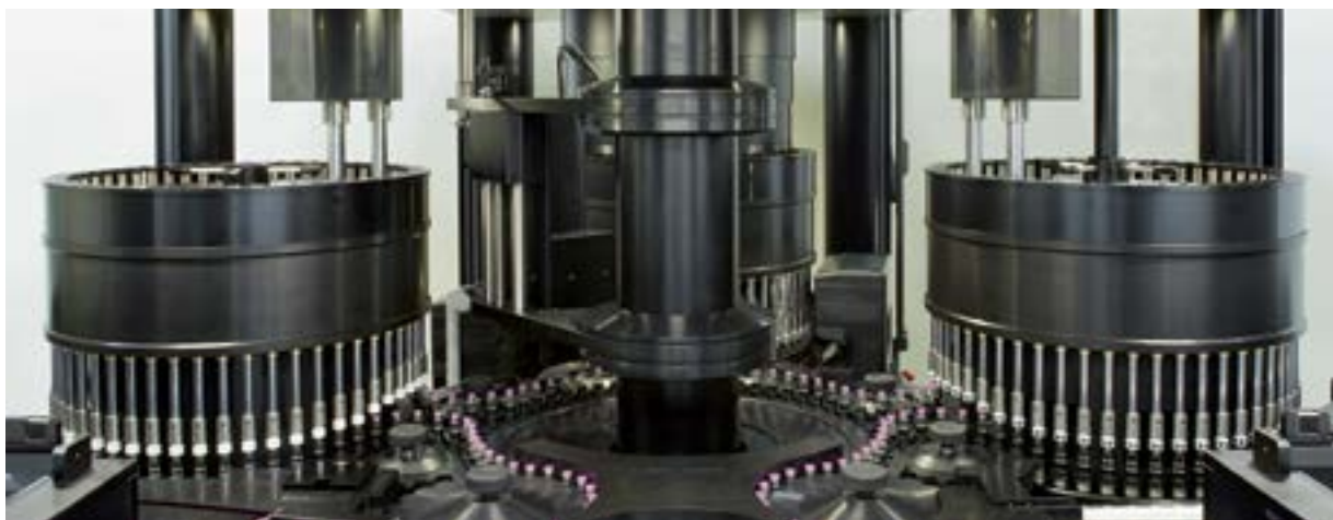
The AIM 8 inspection machine for vials is the first of the new, modular generation of fully automated inspection machines by the Inspection Technology sector of Bosch Packaging Technology.
