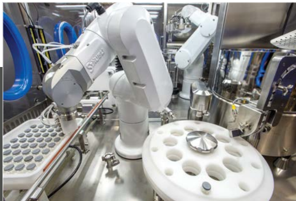
Robots are ideal for when potent compounds need to be handled in isolator containment. They also do not shed particles like humans and achieve ISO 5 standards.
