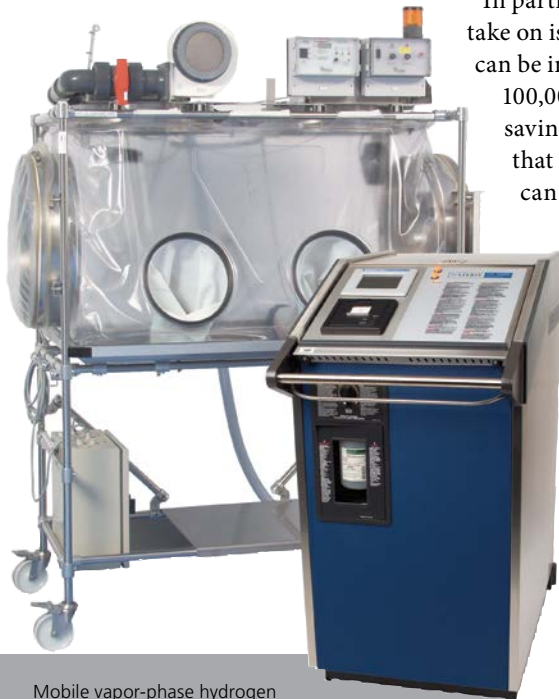
Mobile vapor-phase hydrogen peroxide biodecontamination systems like this one from Steris offer the flexibility users need to support this critical task within aseptic processing environments. (photo courtesy of Steris)
